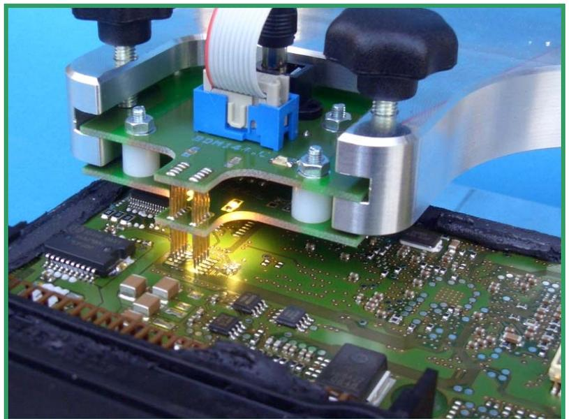
**Pict. C: This way the BDM144 probe contacts the Bosch ME9.0 ECU board..**
