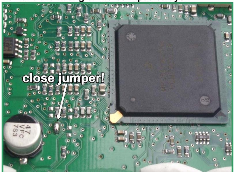
Bild C: This is the location for the required jumper.
