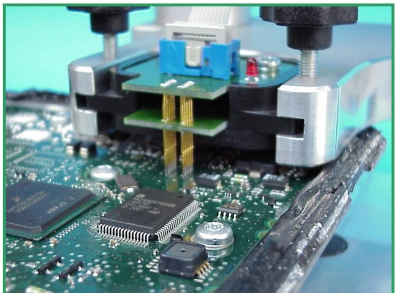
**Pict. C: In this case the BDM144 probe is best suited for contacting the BDM-pads on the PPD1.1.**
