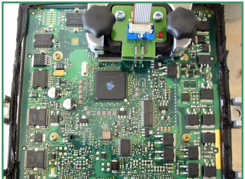
**Pict. C:** The BDM141 probe contacting the BDM pads on the board of the Siemens SID204 ECU
